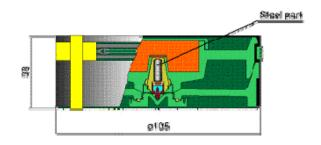
Diameter: 105 mm Height: 38 mm Mass: 183 g 35 g TNT **Explosive charge** Casing: Plastic / rubber Colour: Olive / black Fuse type: Chemical Mode of activation: Pressure Sensitivity: 3 - 15 kps
