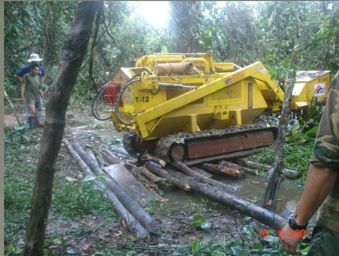
TEMPEST- DIFFICULTIES IN HANDLING IN THE FIELD (Irregular terrain and Muddy conditions)
