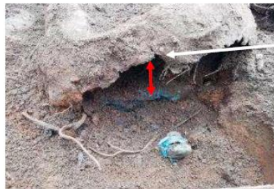
PHOTO 3 | The side of the IED has corroded and some of the (approximately 15kg) explosive substance has fallen out of the container.
