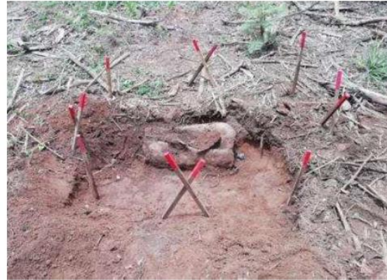
PHOTO 2 | IED after being excavated. Only the bottom part of the item is filled with explosives. The measurement between the explosives and the surface of the ground is more than 20 cm.
